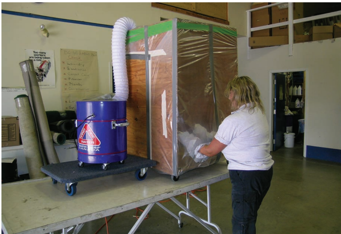
Figure 2. The finished test chamber. The HEPA-filtered air scrubber provides spore-free air prior to starting the tests and purges the chamber following each test.
