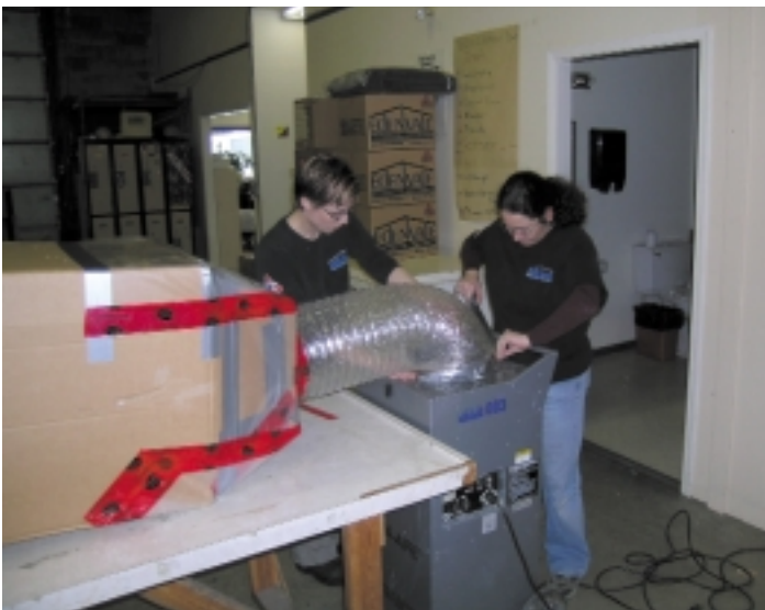
Figure 3 a, b, c: Construction of the unit for treating mold-contaminated paper documents. Note the use of readily available materials and equipment in the construction.
