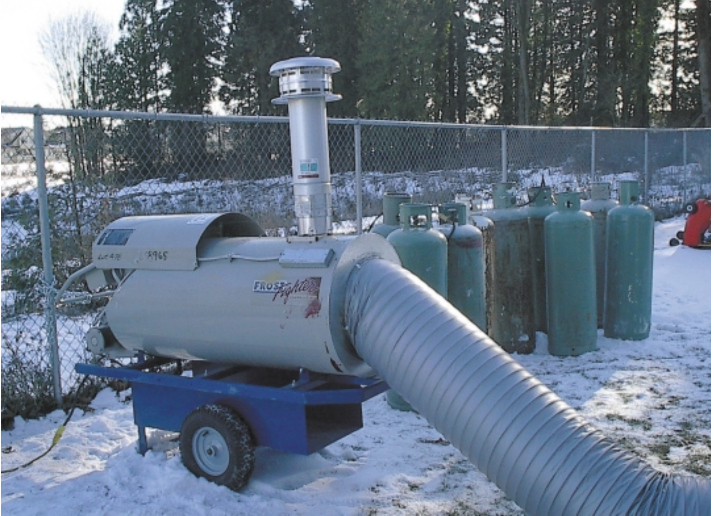
Figure 2. External propane furnace and propane bottles. Note the discharge stack for combustion gases.
