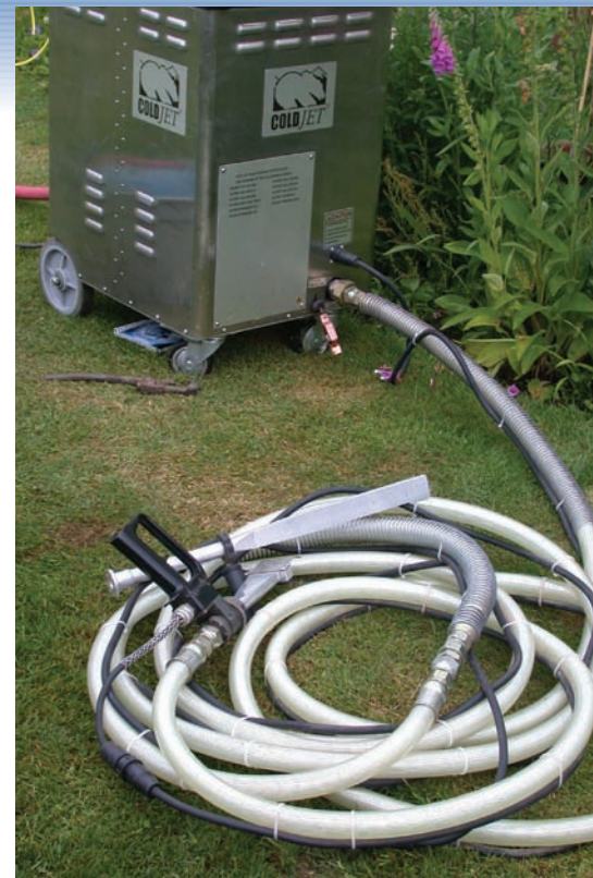
Figure 3. Dry ice auguring machine. Note the clip for attaching to electrical ground. Carbon dioxide pellets transported in compressed air create serious risk of electrostatic discharge. This discharge has sufficient energy to ignite flammable mixtures.
