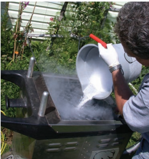
Figure 2. Dry ice handling. Sublimation leading to production of carbon dioxide gas poses the ever-present risk of oxygen deficiency, especially in low-lying areas.
