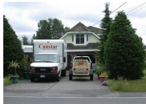
Figure 1. Set-up of the compressor. Note that the location is well-removed from the front of the house to prevent entry of exhaust gases.
